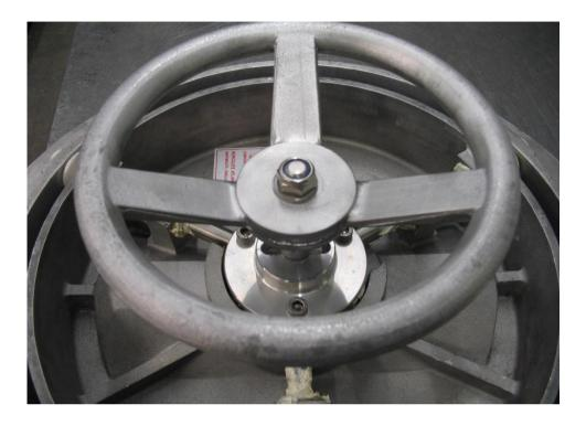
Remove the drive pin from the T - Bar shaft
